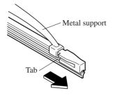
3. Remove the metal stiffeners from each blade rubber and install them in the new blade.
